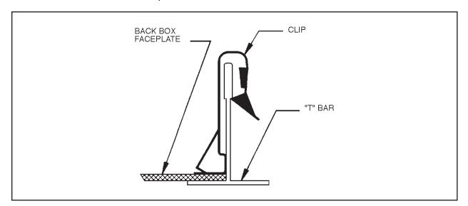
Figure 1. "T-Bar" Clip Installation
